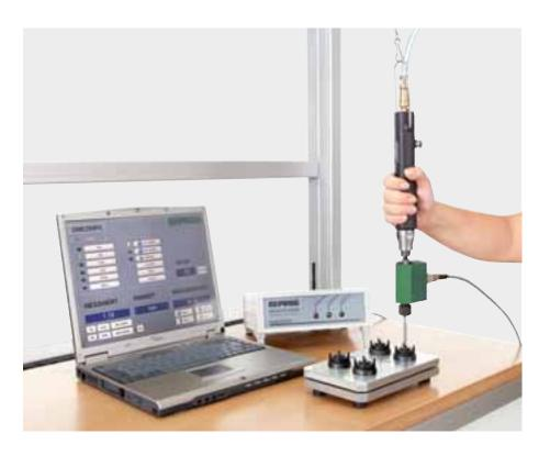
During the actual assembly process, performing torque acquisition and screw-joint analysis is possible. This feature fulfills most or all assembly-process requirements and assures even the highest quality demands.
